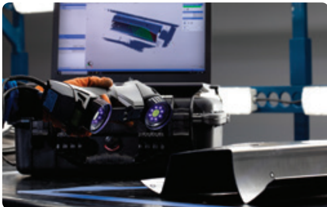
Scanning aluminum for composition.
